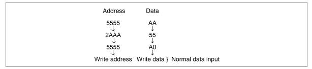
Software data protection mode can be cancelled by inputting the following 6 bytes. After that, this device turns to the non-protection mode and can write data normally. But when the data is input in the cancelling cycle, the data cannot be written.
